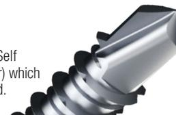
**General Advice on installing MultiONE<sup>®</sup> screws** Fit screw to the driver bit. Place drill tip at fastening location. Apply moderate to firm pressure depending on the material (see over). Commence drilling for the tip to drill a hole. Maintain firm pressure throughout drilling, slowing down as the screw approaches 'home'. Do not over tighten once the screw reaches a flush position.
